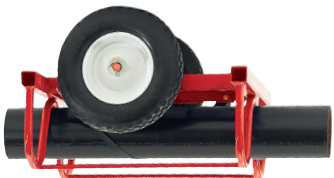
Secure buggy to pipe in the upside down position using the strap supplied
